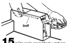
On coin-operated washers, remove the service door of the meter case. Lift the service door up at the back and remove. Carefully insert coin slide with the coin slide extension attached into front opening and secure with the 3/16" mounting bolt from inside the meter case. The coin slide may need to be partially pushed in to insert mechanism in the front opening. Replace meter case top and service door, Insert coin vault with lock and kev.
